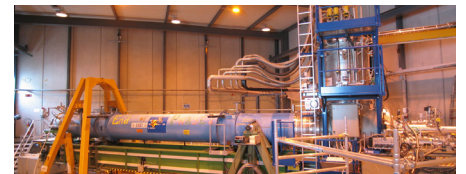
Figure 3: CAST. The telescope magnet (blue) pivots about the right hand side, while the yellow gantry on the left of the picture rolls along a circular track in the floor and raises
